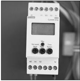
Electronic load limiter This well-proven device will safely stop the winch in the event of an overload.
