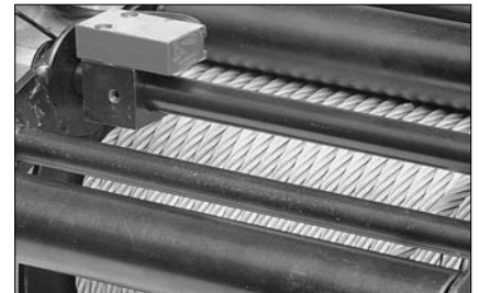
Rope slack switch This device automatically stops the winch when the rope is not taut.
