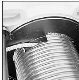
Grooved drum Facilitates correct winding of the first rope layer. Essential for a two-way system.
