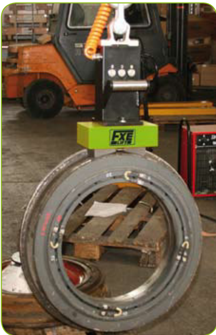
FXE with pole shoe for railway wheels
